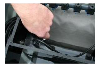
For gravity fed units the sensor is on the clean side of the drum. This sensor is triggered when the micron screen becomes dirty and blocked and the water level starts to drop as not enough water is able to get through.
