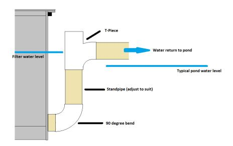
In short runs, the return pipe should be no less than 3" in diameter. For longer runs, 4" is preferable. In the Solum25, 2 x 4" runs would be advisable. In the above diagram, a vertical standpipe governs the height of the water in the filter. A t-piece then returns the water to the pond. A t-piece is recommended as it stops syphoning and/or surging in the return pipe on longer runs.
