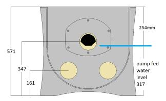
Also in pump fed installations, the filter needs to have the water level set at this height by an external standpipe return. The following diagram shows this layout –
