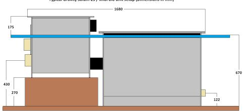
Typical Gravity Solum 25 / Midi bio unit setup (Dimensions in mm)
