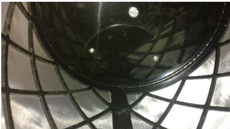
If you need to bypass the drum, for instance if you are treating for flukes, there is a bypass plate that can be removed from inside the drum itself and is secured by 2 self tapping screws. This is accessed by removal of the waste tray.
